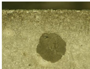
Fig. 1. Microstructure of the surface layer in ADI sample after cyanide case hardening; Magnification x750
